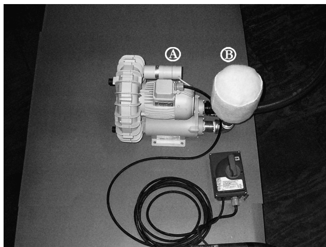
FIG. 1. Air pump delivering filtered air to wash basin. (A) Air pump. (B) Filter.
