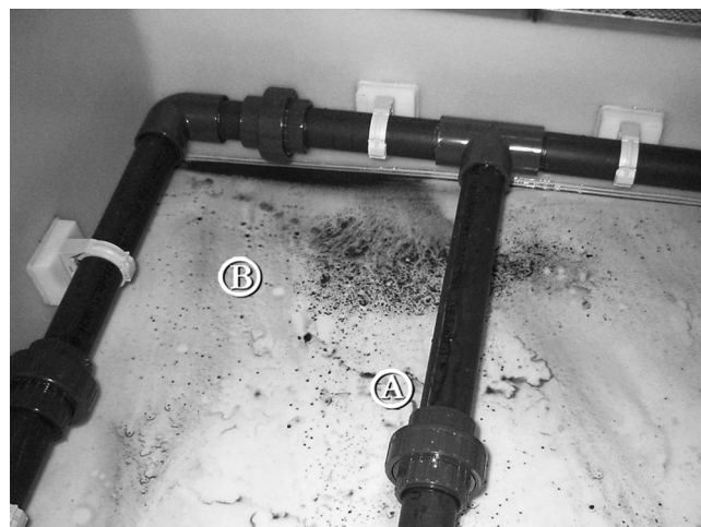
FIG. 3. Washing container. (A) Air delivery system. (B) Soil/debris after one washing of seeds.
