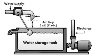
An approved Air Gap (AG) is a physical separation between the free-flowing discharge end of a potable water supply pipeline, and the overflow rim of a storage tank. This separation distance must be at least 2 times the discharge pipe diameter with a minimum of one (1) inch.
