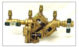
A Reduced Pressure Backflow Assembly (RP) is designed to prevent backflow. The RP assembly consists of two independent springloaded check valves separated by a springloaded differential pressure relief valve, two shutoff valves and four test cocks. Air Gap (AG)
