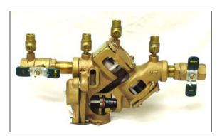
A Reduced Pressure Backflow Assembly (RP) is designed to prevent backflow. The RP assembly consists of two independent spring-loaded check valves separated by a spring-loaded differential pressure relief valve, two shutoff valves and four test cocks.
