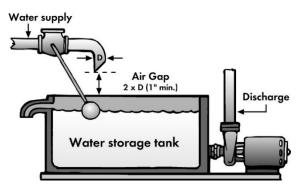
An approved Air Gap (AG) is a physical separation between the free-flowing discharge end of a potable water supply pipeline, and the overflow rim of a storage tank. This separation distance must be at least 2 times the discharge pipe diameter with a minimum of one (1) inch.
