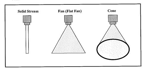
Some special purpose nozzle tips or devices produce special patterns. These include raindrops, flooding, and others that produce a wide-angle fan or cone-shaped patterns. Some special purpose nozzles are manufactured for a specific purpose, such as drift reduction or air-induction nozzles.
