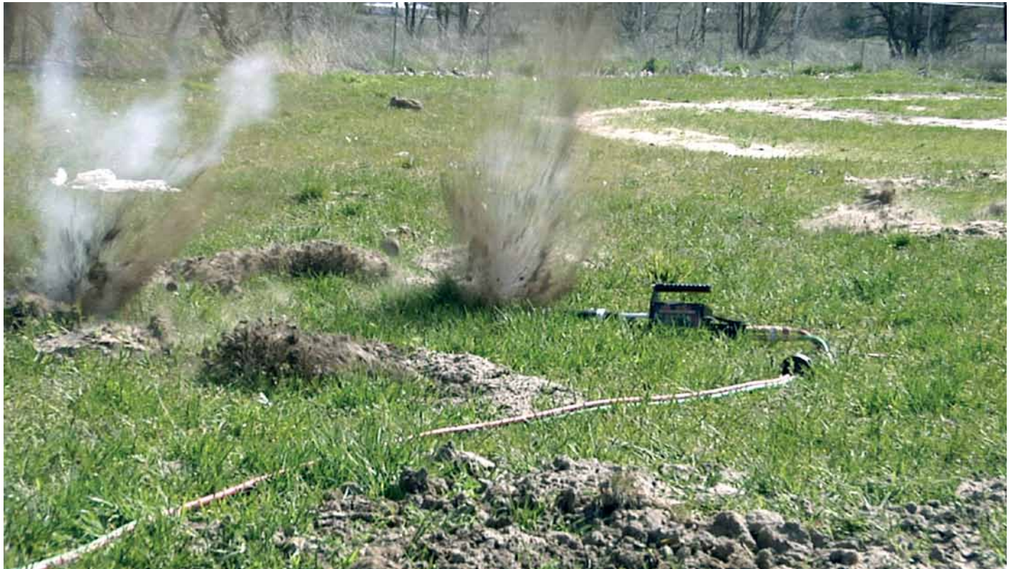
Figure 23. Gopher control in a large infestation using the Rodenator. The Rodenator uses a mixture of oxygen and propane to kill gophers and collapse tunnel systems. Photo reproduced courtesy of Meyer Industries, Emmett, Idaho.
