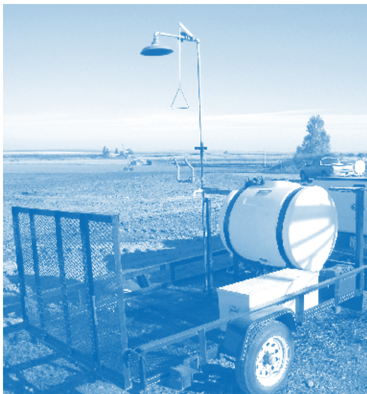
Portable decontamination unit
