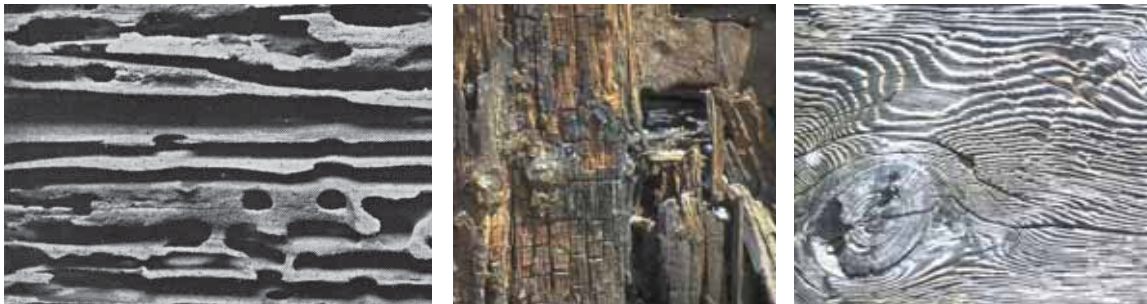
Figure 1. Wood products that are in contact with the ground or exposed to weather can be damaged by a variety of damaging insects (left), fungi (middle), and marine borers, as well as by the weather itself (right).
