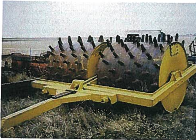
Figure 10D-18 Longer style of teeth preferable for compacting soils for clay liner
